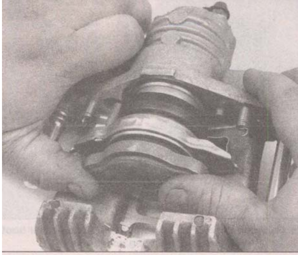
3.32 With the piston, actuating collar retainers and dust boots and clamp rod in position, square to the bore, use your thumbs to push the piston into the caliper
