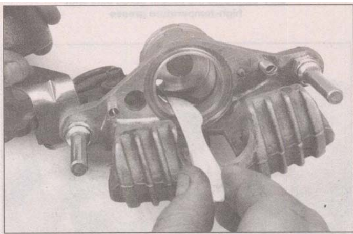
3.25 Use a wood or plastic tool to remove the piston seal from the bore
