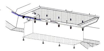
Have the new switch ready to install, with a small amount of low-strength sealer like blue Locktite.
