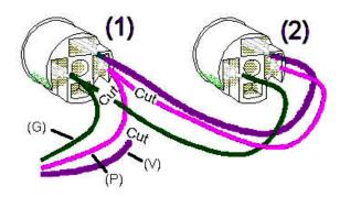
Use a small jeweler's screwdriver to remove the green and pink wire terminals from the remaining socket. Push the flat blade into the small slot adjacent to the blade. It will flatten a retaining tab so that the terminal can be removed. Alternately, if you have a good crimper, you can cut the wires and put on a new terminal end included with the update kit.
