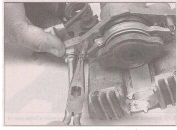
3.20 Remove the springs from each end of the parking brake collar
