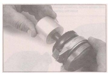
3.30 Lubricate the clamp rod bushing with the supplied lubricant, then slide the piston onto the clamp rod bushing
