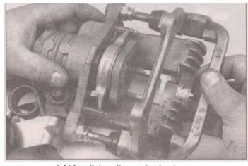
3.36 Install the caliper anchor bracket
