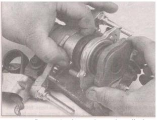
3.22 Remove the clamp rod, actuating collar boot retainers, actuating collar boots, actuating collar and piston as a single assembly
