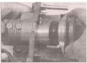
blowout all the passages in the caliper housing and pleeder valve.
