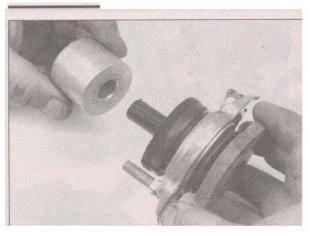
3.23 Slide the piston off the clamp rod bushing
