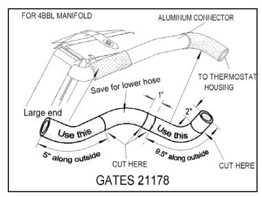
The long leg of the aluminum connecting tube goes toward the radiator.
