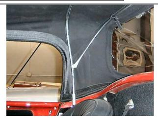
Note the strap that keeps the rear brace in position just above the window line.
