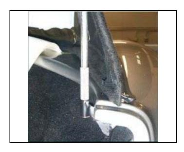
Assemble the rear bow halves together. Turn the knurled adjusters all the way into the ends of the bows.
