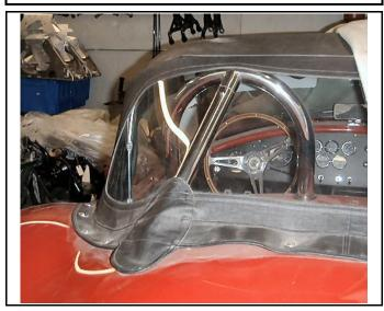
Beginning at the center, carefully un-tape a portion of the top fabric from the windshield. Glue a portion of the top fabric to the front vertical face of the channel with contact cement. Do not apply the glue to the top of the front bow, only to the front surface. Work from the center to the sides until the entire top surface is glued.
