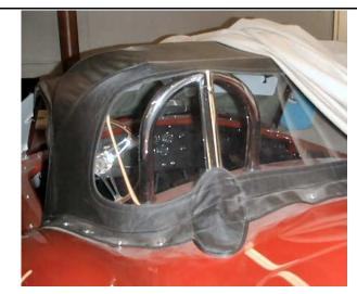
The roll bar rear brace requires an addition that goes into the window.
