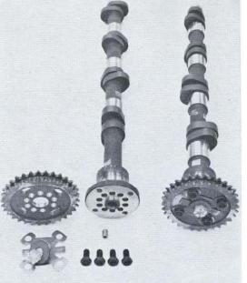
ABOVE LEFT - Around and around and up and down we go, following the motion of the OHC chain drive. Shorter chain is primary power source tapped from crankshaft. Stub shaft fits into spot normally held by camshaft, drives oil pump, distributor. Cam speed is 1/2 crank.
